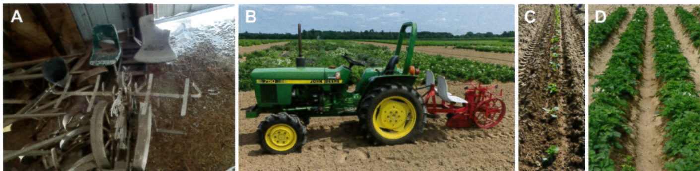
The finger transplanter is shown before (A) and after (B) refurbishment. Mechanically transplanted seedlings are pictured on the day of transplanting (C) and one month later (D).
